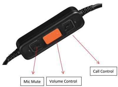
Check the operation by making a call on the softphone via Sirius USB Headset. Press the mic mute button, the LED will glow in red and verify whether the caller cannot hear your voice. To release mic mute, press the mic mute button again.
